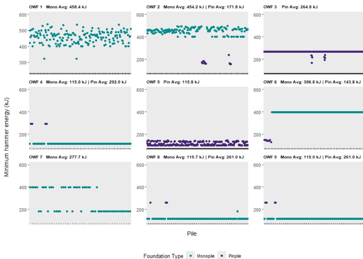
Figure 18. Minimum hammer energy per pile during the soft-start (with soft-start duration as defined by the MMMP).
