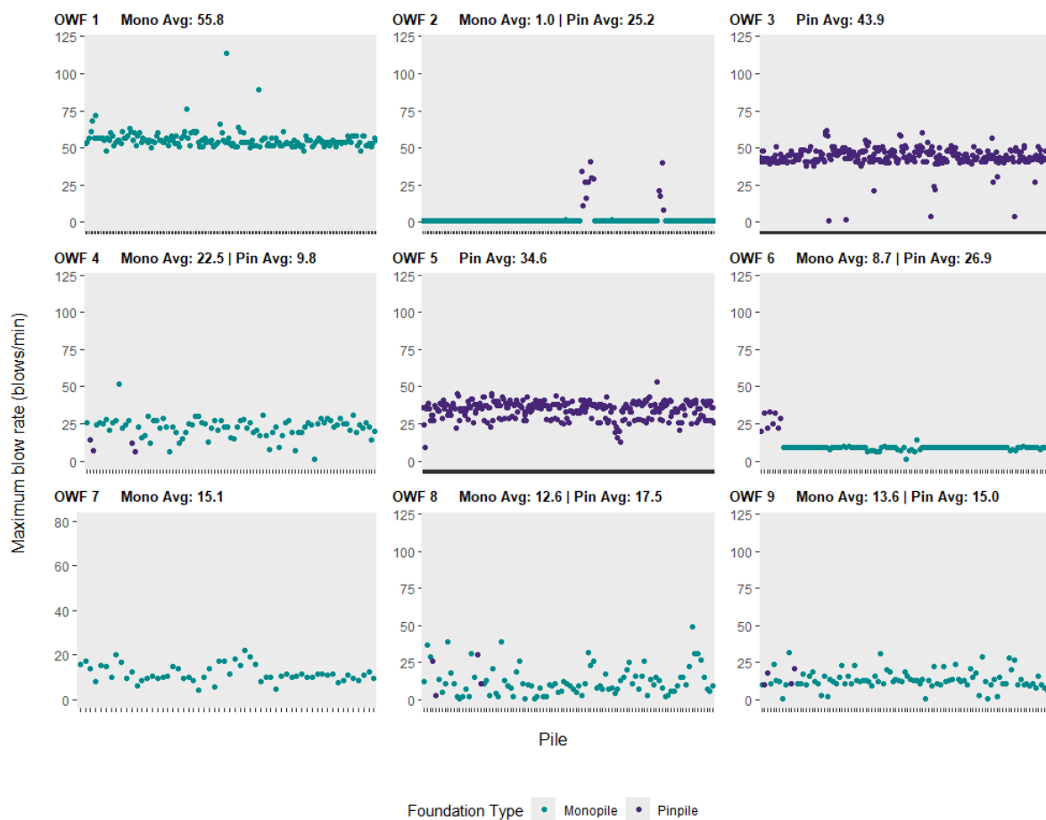
Figure 22. Maximum blow rate during the soft-start for each pile (with soft-start duration as defined by the MMMP).
