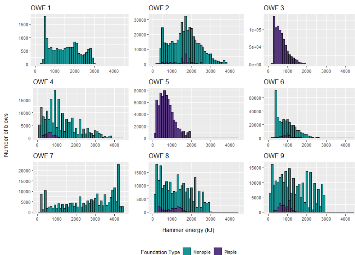
Figure 5. Box plots of the hammer energies used during piling (including the soft-start) across OWF 1-9.
