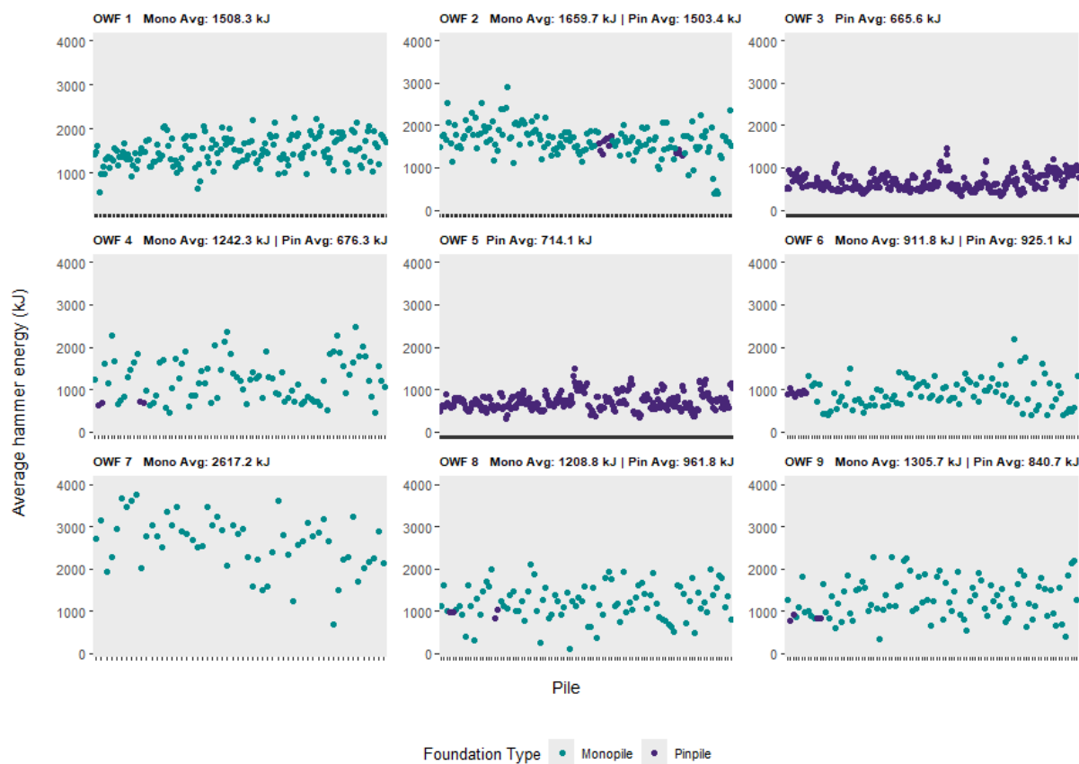
Figure 19. Average hammer energy per pile across the entire pile installation.
