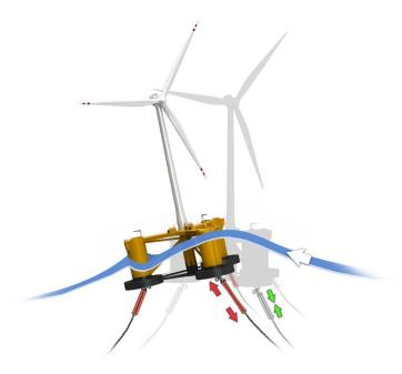
The IMS reduces peak loads on the platform by extending in length and increasing stiffness through the wave cycle
