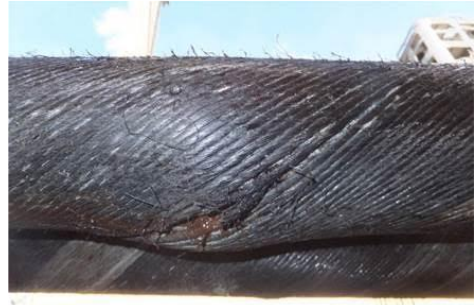
Figure 21: Cable thermal degradation (PeakWind)
