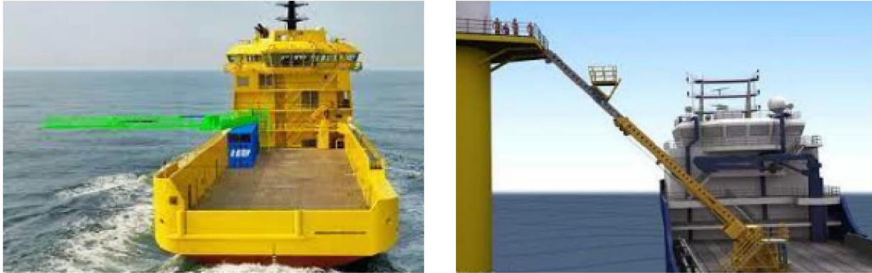
Figure 14: Examples of a L-bow (left) and Z-bridge (right) W2W system. 14
