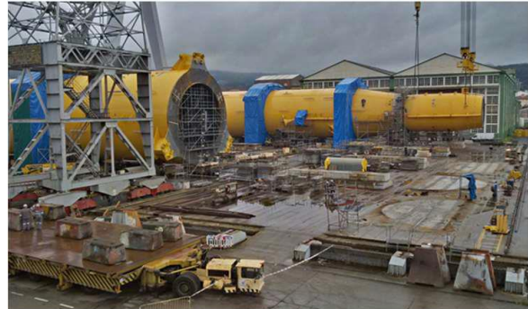
Figure 17: Floating foundation fabrication (Navantia)
