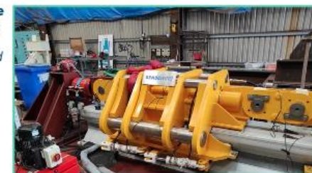
RNA carriage lower clamp assembly: Function and load testing
