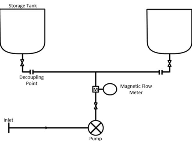
Figure 4 - BV Dairy Mascarpone Mixing Circuit
