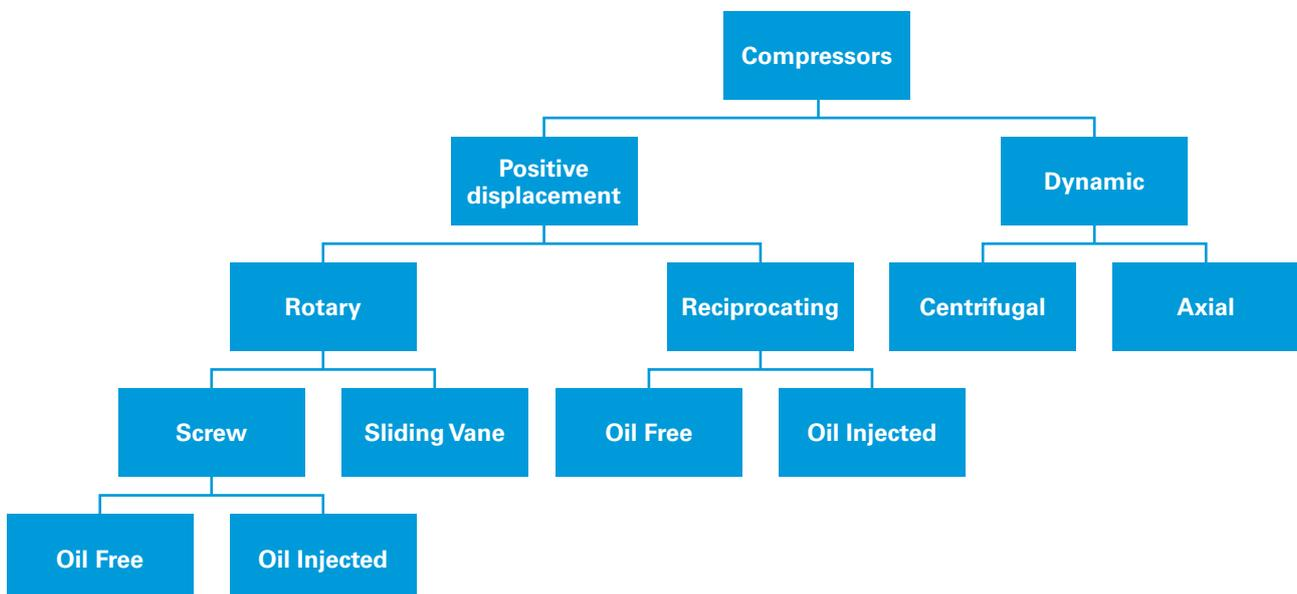
The majority of compressors currently being used on general purpose compressed air systems are oil injected screw machines.
