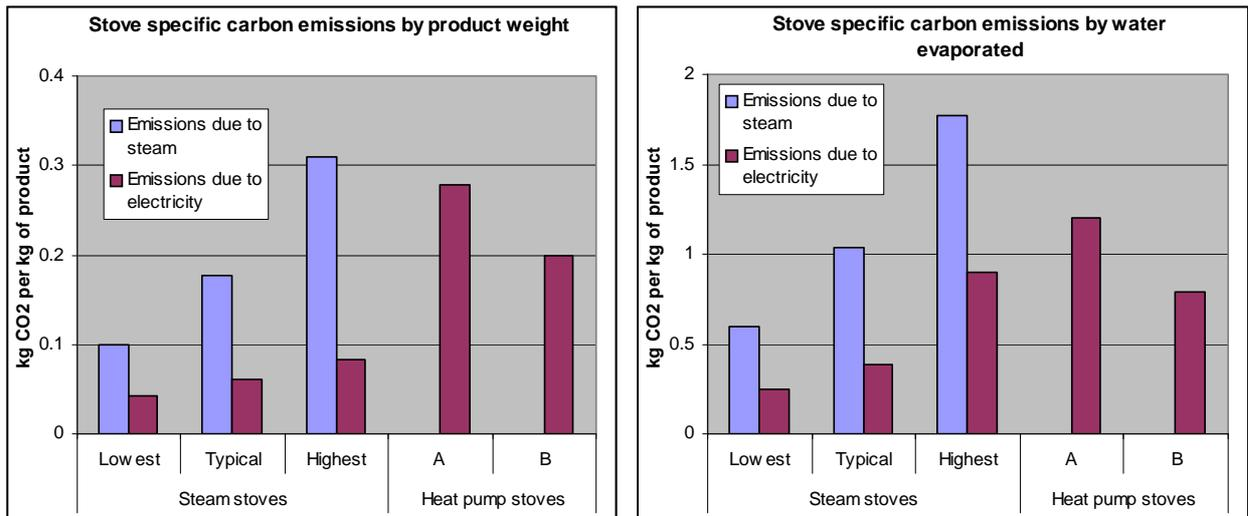
**Figure 11: Comparative CO<sub>2</sub> emissions from steam and heat pump stoves**
