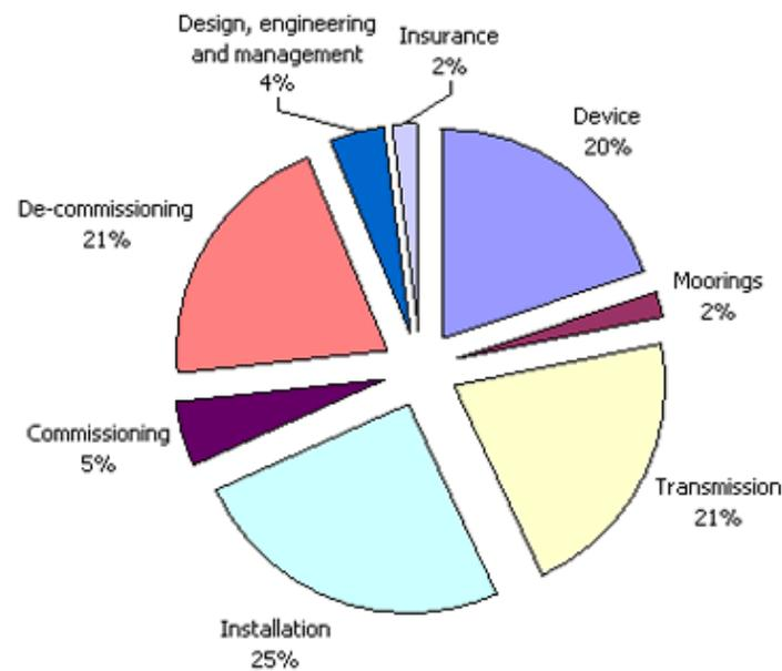
**Figure 1c: Capital cost breakdown for installation of a particular wave energy device in a wave farm of a certain size**
