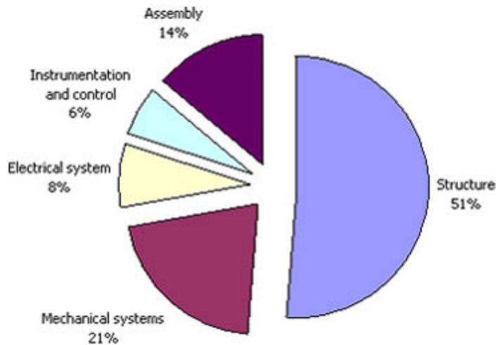
Figure 1b: Capital cost breakdown for installation of a particular wave energy device as one single unit
