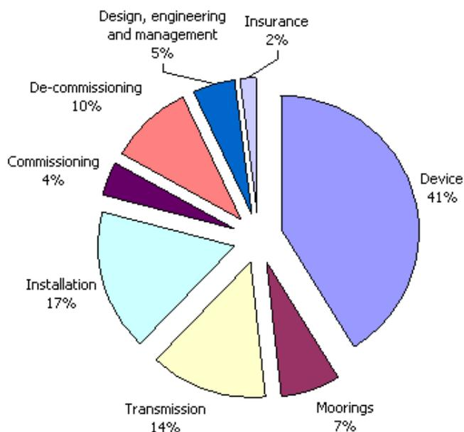
**Figure 1d: Capital cost breakdown for installation of a particular tidal stream energy device in a tidal stream farm of a certain size**
