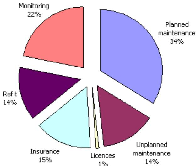
**Figure 2b: O&M cost breakdown for a wave farm of a certain size involving one particular wave energy device**
