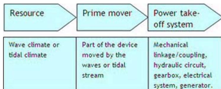
Because of the many ways that marine renewables devices can be configured, their performance characteristics vary widely. To understand performance characteristics in detail, it is necessary to look closely at specific device designs. However, it is possible to make general observations about the performance characteristics of wave energy and tidal stream devices and identify requirements for high performance that are common to many design variants.
