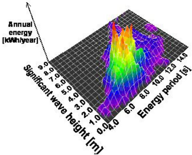
Figure 7: Example wave energy device power surface with distribution of wave energy with wave height and wave period superimposed.
