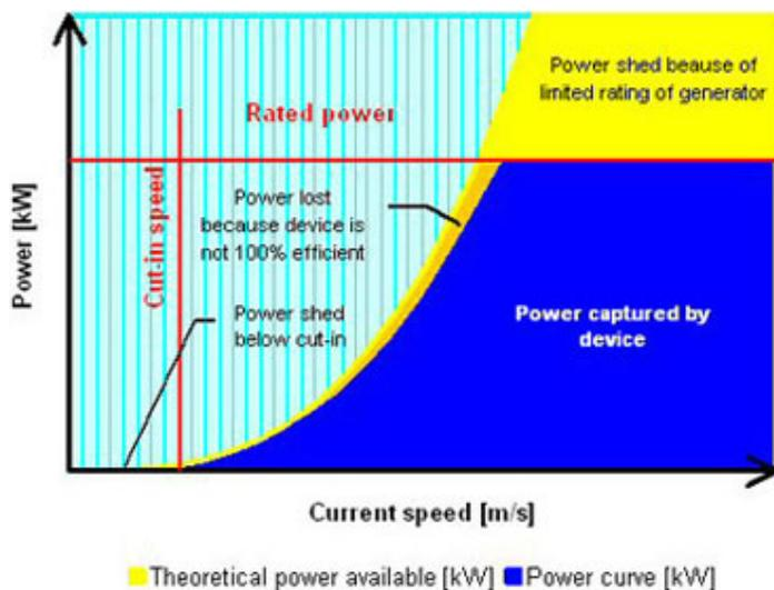
**Figure 3: Example wave energy device power surface highlighting conditions where no power is generated**
