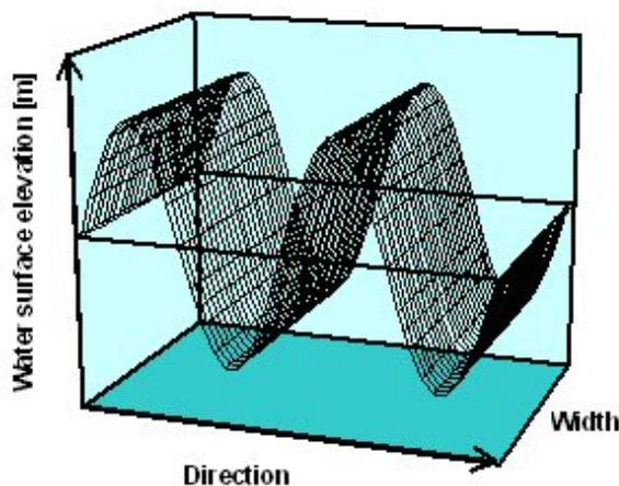
**Figure 2a: Several sinusoidal wave components with different amplitudes and wavelengths**
