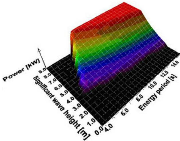
Figure 11: Combination of device power surface and sea scatter diagram
